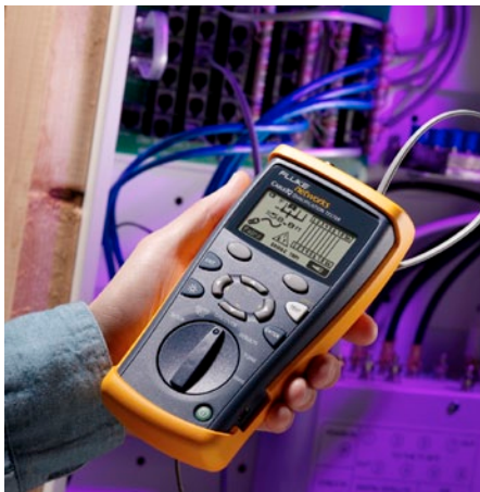
Qualification tools will tell you what services can be successfully deployed on a given link. This example shows a link suitable for VoIP, 10BASE-T and 100BASE-TX, but unacceptable for 1000BASE-T.
